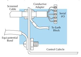
grounding one end, which primarily originated as a result of trying to reduce hum in audio systems, is no longer applicable to the complex industrial environment. Shielded cables are also efficient emitters of RF noise from the CPU system, and can interact in a parasitic manner in networks and between multiple sources of interference.
