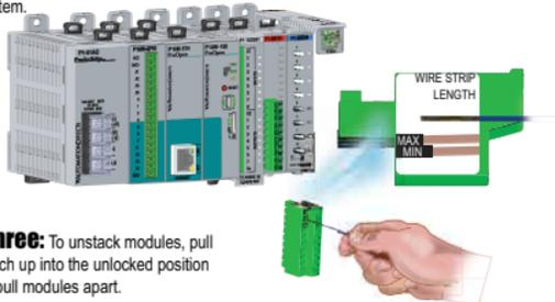
**Step Three:** To unstack modules, pull locking latch up into the unlocked position and then pull modules apart.
