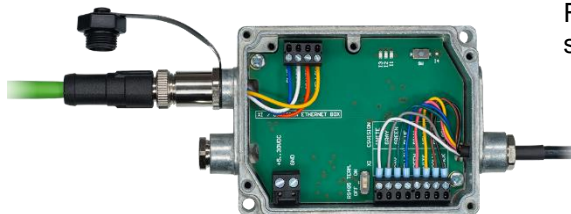
Figure 1: Optris Ethernet TCP/IP / Modbus TCP communication interface board
