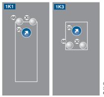
05 = switching distance adjuster 30 = switching status indicator / contamination warning 68 = supply power indicator
