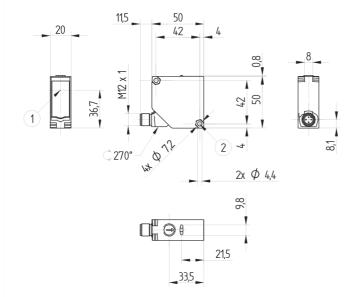
1= Optical axis M4 screw = 0.5 Nm Potentiometer = 40 Nmm Dimensions specified in mm (1 mm = 0.03937")
