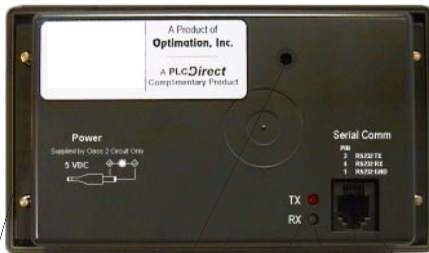
Power Receptacle Location LED Display Intensity Adjustment Control TX LED (Red) RX LED (Green) RJ12 Connection
