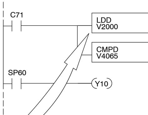
This rung loads the value from V2000 & V2001, and compares it to the value in V4065 & V4066.
