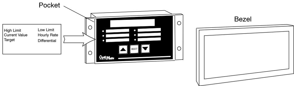
Remove the bezel from the module by unsnapping the four plastic tabs which hold the bezel to the module frame. Locate the pocket, and carefully slide the labels into place. Re-attach the bezel by snapping the bezel onto the case.
