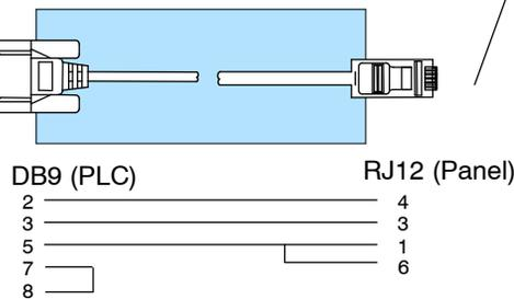
The drawings on this page are for cables which **are not** supplied by **Automationdirect.com**. Use the drawings to make your own cable. We recommend using a 22 AWG or larger shielded cable.
