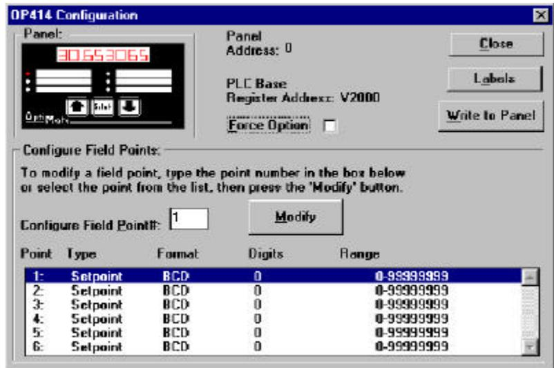
Open the Field Point Configuration window below by double-clicking on the Point selected or clicking Modify with the Point selected.
