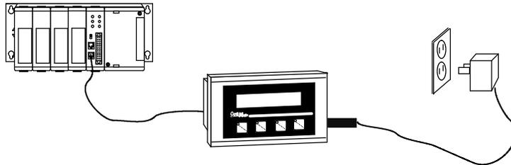
**Operation Using a DL05, DL105, DL205, or Top Port of DL405 CPU: 5 VDC Power Supply Not Required**
