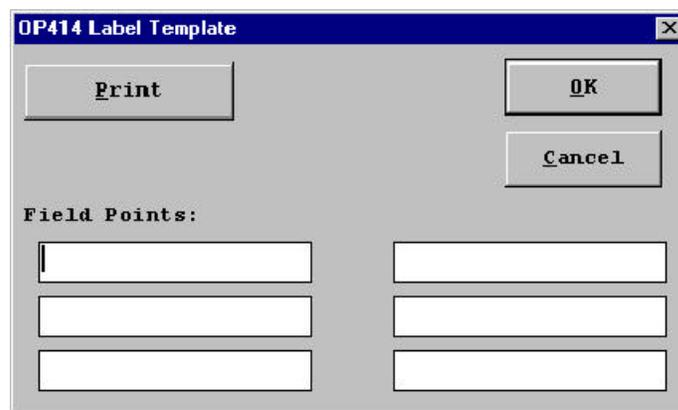
4. The OP-414 Label Template appears. Type in the label text for all six Field Points. Press **OK** to save the labels.
