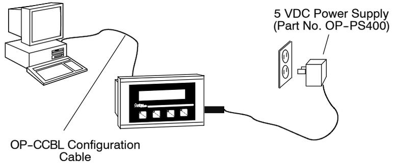
**Operation Using a D3-340, D3-350, D3-330 w/DCU, Bottom Port of DL405 or Allen-Bradley CPU: 5 VDC Power Supply Required**
