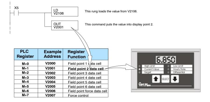
**Reading a Setpoint** The OP-413 continuously updates the registers of all setpoints with each setpoint's current value. To read a setpoint, simply access the register(s) that correspond to each setpoint. The data can be copied to another register for manipulation or it can be accessed in its field point register(s).
