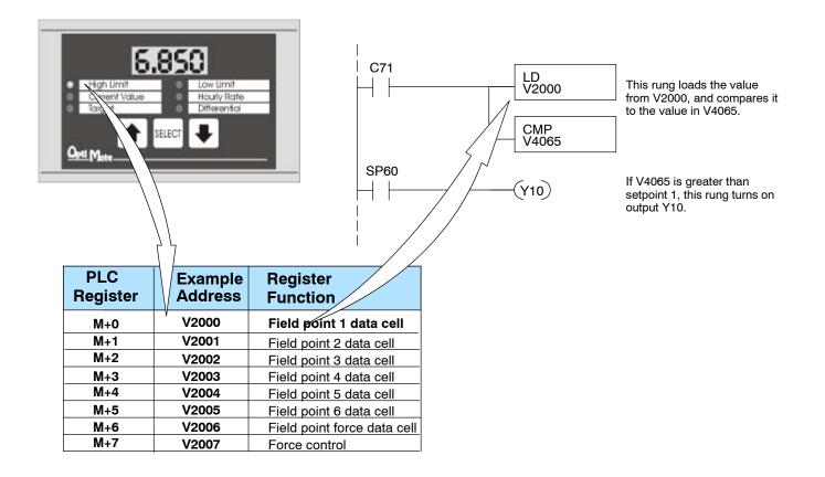
**Forcing Setpoints** The OP-413 allows you to force a setpoint to a value from the PLC. In order to force a setpoint to a value, place the value into register M+6. Then set the FSP and bit(s) corresponding to the setpoint(s) to be forced. When the panel has completed the force operation, it clears registers M+6 and M+7.
