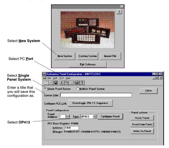
Step 5Select Configure PLC Link - Here is<br/>where you define protocol items such<br/>as PLC address, baud rate and parity.<br/>Enter the appropriate parameters for<br/>your PLC. The following table provides<br/>the necessary information for most<br/>DirectLogic controllers. For other PLC<br/>families, reference that product's user<br/>manual to determine the port<br/>communications capabilities.
