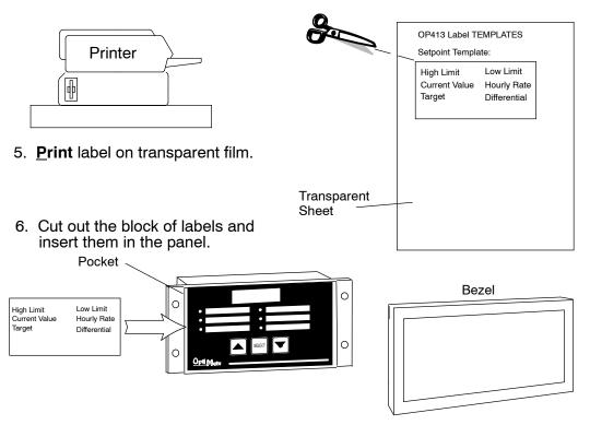
Remove the bezel from the module by unsnapping the four plastic tabs which hold the bezel to the module frame. Locate the pocket, and carefully slide the labels into place. Re-attach the bezel by snapping the bezel onto the case.
