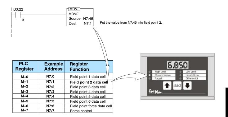
**Reading a Setpoint** The OP-413 continuously updates the registers of all setpoints with each setpoint's current value. To read a setpoint, simply access the register that corresponds to each setpoint. The data can be copied to another register for manipulation or it can be accessed in its field point register.
