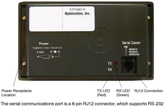
SerialThe serial communications port is a 6-pin RJ12 connector, which supports RS-232Communicationsinterface wiring. This port is used for communications between the OP-panel and<br/>PLC, as well as for programming your panel configurations.
