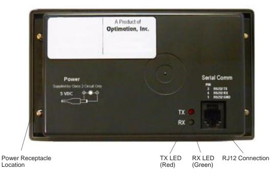
Serial<br/>CommunicationsThe serial communications port is a 6-pin RJ12 connector, which supports RS-232<br/>interface wiring. This port is used for communications between the OP-panel and<br/>PLC, as well as for programming your panel configurations.
