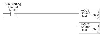
Load message #3 for top line display register m+0.
