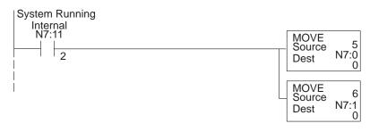
Load message #5 to top line display register m+0
