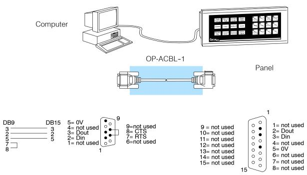
This cable must be used to <u>configure</u> the panel.
