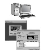
Step 4: Configure<br/>the Panel to Work<br/>with your PLC<br/>(Pages 15)After setting a DIP switch on the rear of the panel<br/>and attaching the programming cable, you are<br/>ready to configure your panel. The simple and<br/>easy-to-follow screens make configuration a<br/>painless process.
