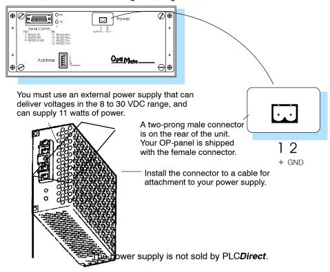
NOTE: The majority of the power consumed by the panel is used in the LED light bars. The current drawn by the panel is shown in the specifications below. Do not attempt to use the 24 volt power output of the CPU and/or the PLC base instead of using a proper external power supply. With all the lamps lit, the current drawn by this panel will exceed the current rating of the CPU or base and could damage your equipment.
