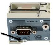
NOTE: The grounding screw below the D-Sub connector must always be connected to earth ground.
