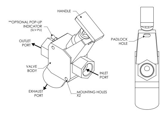
\*\*INDICATOR EXTENDED WHEN PRESSURE IS PRESENT BEYOND THE OUTLET PORT. TO VERIFY INDICATOR IS WORKING - USING FINGER, PUSH THE RED BUTTON. IF PRESSURE CAN BE FELT, THE INDICATOR IS WORKING.
