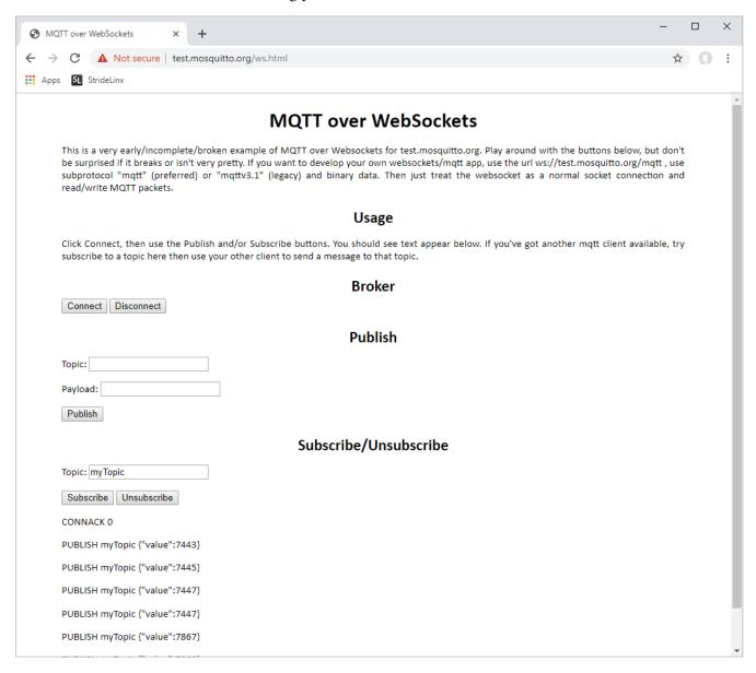
If the PUBLISH messages are showing up on the screen, the MQTT functionality and network path are correctly configured.
