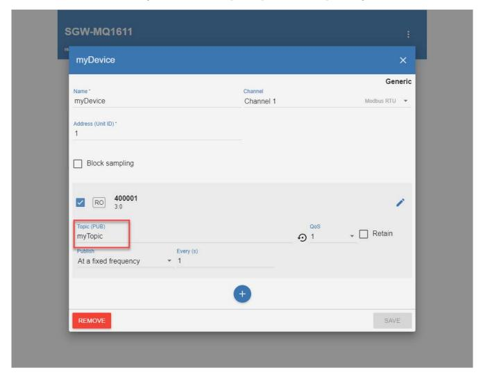
Once this setup has been saved to the gateway, we can go to the "test.mosquitto.org/ws.html" URL to check and see if our gateway is publishing data to the Broker.
