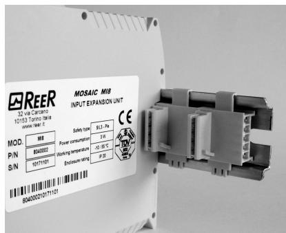
3. Fasten the units to the rail, arranging the contacts on the base of the unit on the respective connector.
