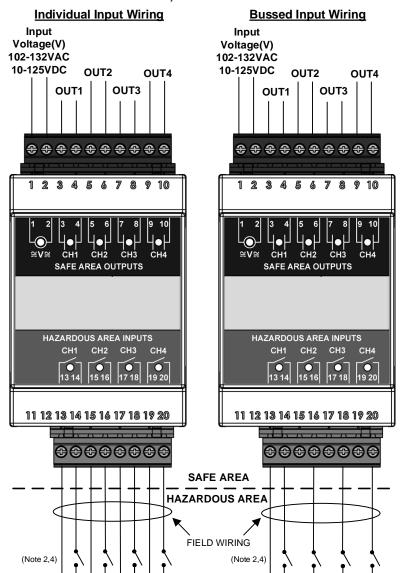
(Separate terminals are provided for connection of two conductors per channel. Use of all channels is not required. Individiual, bussed, or a combination of input wiring configurations may be used.)
