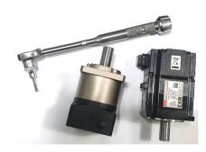
① Check to see if the gearbox is the proper one for the motor you have Clean the combining surface.
