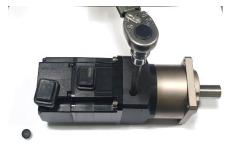
Tighten the shaft collar bolt with torque wrench to the torque specified in the 'Shaft collar bolt'table.
