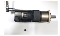
Tighten the bolts with torque wrench to the torque specified in the 'Motor installation bolt'table.
