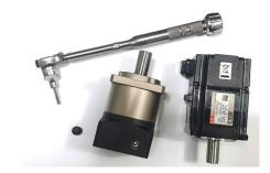
Remove the plug from the gearbox adapter's clamp hole. Loosen the shaft collar bolt through clamp hole on Gearbox adapter.
