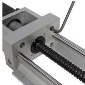
28) Install the second spacer sleeve onto the machined end of the ball screw at the flanged mounted bearing support unit.
