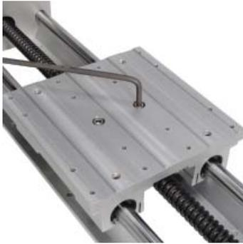
31) Slide the motor, motor mount, coupler assembly onto the ball screw. Install the four motor mounting screws using a 5/32" hex key.
