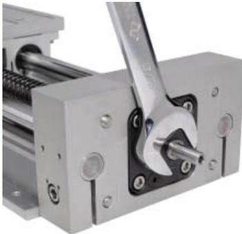
32) Tighten the drive coupler collar lock using a 2.5mm hex key to clamp onto the ball screw.
