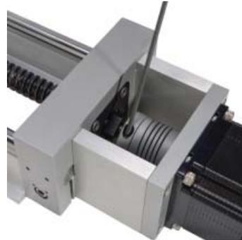
30) Tighten the two set screws on the bearing locking nut using a 1.5mm hex key.
