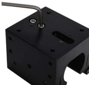
32) Install the sensor mount brackets at both ends. Note the orientation of the sensor flags on the carriage bottom. Secure using a 0.050-in hex key on the set screws.
