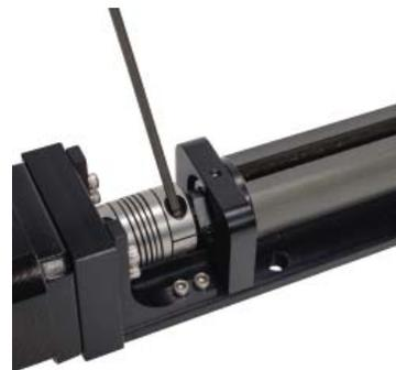
34) Install the motor bracket and motor flange to the base using a 3/32-in hex key. If a motor is present, secure the motor shaft to the coupler using a 2mm hex key.
