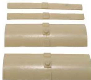
18) Lay the carriage on its side and insert one of the two larger slide bushings into the housing. You will feel a positive snap when it falls into correct placement. Now place the second large slide bushing into the carriage so that it snaps into place. A little grease on the back side of the bushings will help to hold it in place until the slide tube is engaged.
