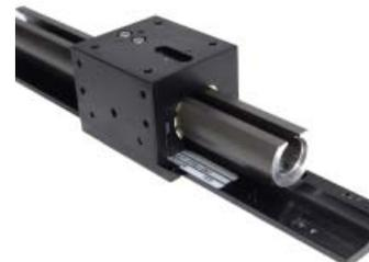
20) Once the carriage is on the slide tube, vigorously move the carriage to seat the slide bushings and insure alignment. Slide the carriage to the drive end of the tube and expose as much of the inside of the carriage as possible. Do not slide the carriage off the end of the tube.
