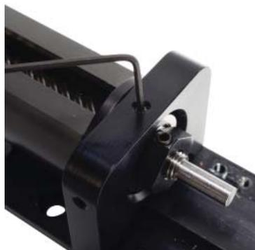
33) Install the new coupler onto the lead screw using a 2mm hex key.
