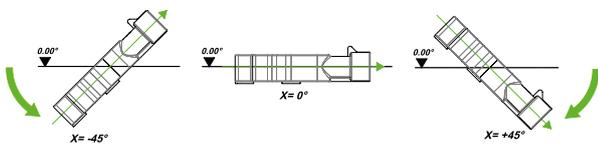
DUAL AXIS TILT SENSOR (XY) - Y AXIS
