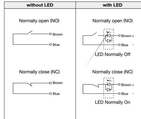
When using the switches with LED option, limit the current below 10mA.
