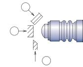
When sliding, be sure that rotational torque is not applied to the plunger shaft.
