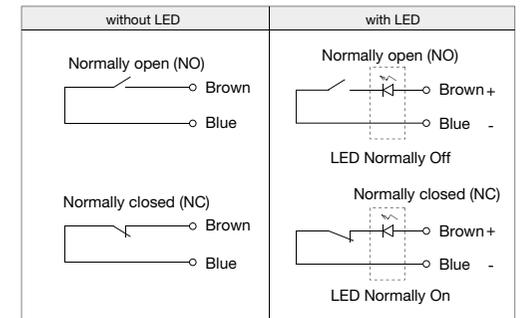
When using the switches with LED option, limit the current below 10mA.
