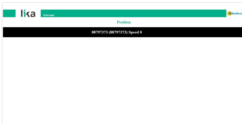
Figure 5 - Encoder position and speed page
