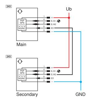
The example shows an application using two digital sensors. In this case, pins 2 and 4 on the main can be used to set the switching points in relation to the calculated difference or thickness. Two analog sensors or a combination of digital and analog sensors can also be used. In this case, the calculated thickness can then be tapped on the main sensor's analog output as an analog signal.
