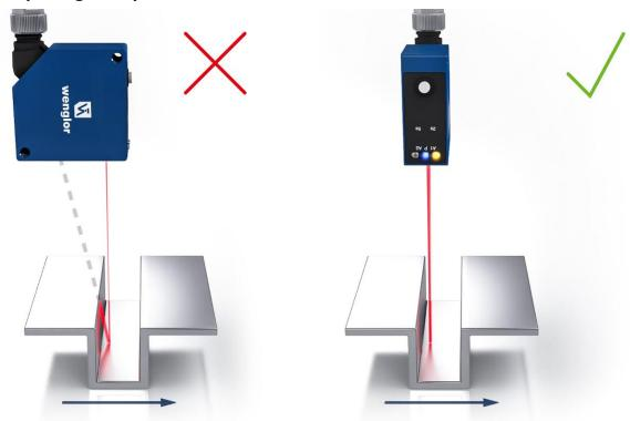
If measuring directly next to steps/edges/depressions, make sure that the receiving beam is not covered by the step/edge. The same applies when measuring the depth of gaps and holes.
