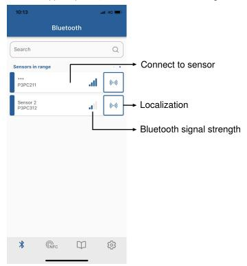
If too many sensors of the same type are fitted within the Bluetooth range, the sensor's supply voltage LEDs can be switched to flashing green by pressing the "Localization" button. This simplifies identification.
