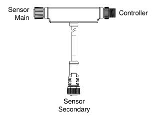
The connections of the adapter can be extended with connection cables. Please note that 5-pin connection cables must be used for the connections of the sensors.
