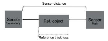
We recommend positioning the sensors in such a way that there is no area between the sensors which is not covered by the sensors' measuring range (Fig. 1 and 2). If this is the case, the object to be measured must be wider than the area not covered (Fig. 3).
