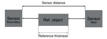
We recommend positioning the sensors in such a way that there is no area between the sensors which is not covered by the sensors' measuring range (Fig. 1 and 2). If this is the case, the object to be measured must be wider than the area not covered (Fig. 3).
