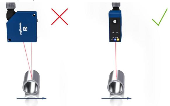
With round, glossy surfaces, the sensor should be positioned on an axis with the round object in order to avoid reflection.
