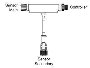
The connections of the adapter can be extended with connection cables. Please note that 5-pin connection cables must be used for the connections of the sensors.
