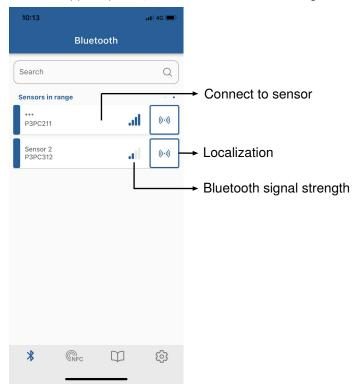
If too many sensors of the same type are fitted within the Bluetooth range, the sensor's supply voltage LEDs can be switched to flashing green by pressing the "Localization" button. This simplifies identification.
