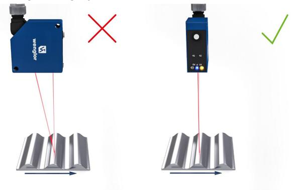
When measuring a moving object, the object must be able to move transversely to the sensor. This prevents shadows and direct reflection to the receiver.
