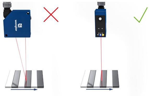
When oriented correctly, the influence on measuring accuracy is minimal. When oriented incorrectly, the different reflectivity of the various colors will result in deviations.
