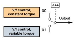
• The built-in V/f curves are oriented toward developing constant torque or variable torque characteristics (see graphs below). You can select either constant torque or reduced torque V/f control.
