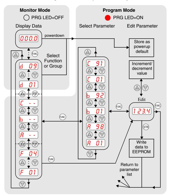
The navigational map shows the relationship of all resources of the inverter in one view. In general, use the key to move left and right, and the (arrow) keys to move up and down.
