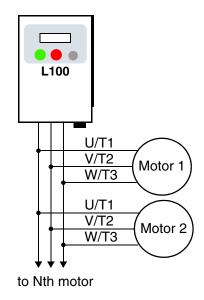
• The wiring for the motors must be permanently connected in parallel (do not remove one motor from the circuit during operation).
