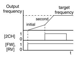
In the graph shown above, the [2CH] becomes active during the initial acceleration. This causes the inverter to switch from using acceleration 1 (F\_02) to acceleration 2 (A\_92).
