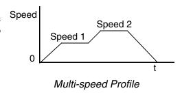
tively, the selected speed is infinitely variable across the speed range. You can use the potentiometer control on the keypad for manual control. The drive accepts analog 0-10V signals and 4-20 mA control signals as well.
