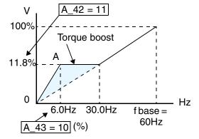
parameters A\_42 and A\_43. The manual boost is calculated as an addition to the standard straight V/f line (constant torque curve).
