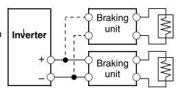
Use one BRD-EZ2 braking unit for the braking torque listed in the following table.
