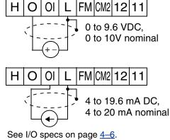
250 Ohms. Attach the cable shield wire only to terminal [L] on the inverter.
