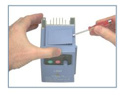
The top housing cover is held in place by four locking tabs. To remove the cover, squeeze two corners together and push a small screwdriver under one side as shown, while pulling upward. Hold the screwdriver at the angle shown, and DO NOT push the screwdriver or any object through ventilation openings and into the inverter.
