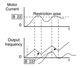
When the inverter detects an overload, it must decelerate the motor to reduce the current until it is less than the threshold. You can choose the rate of deceleration that the inverter uses to lower the output current.
