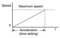
ending frequencies. However, the slope is constant, corresponding to the full-scale accel or decel time setting. For example, the full-scale acceleration setting (time) may be 10 seconds—the time required to go from 0 to 60 Hz.
