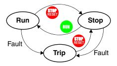
either case, you can clear the fault by pressing the Stop/Reset key. Additionally, you can clear the inverter's cumulative trip history by performing the procedure "Restoring Factory Default Settings" on page 6–8 (setting B\_84=00 will clear the trip history but leave inverter settings intact).
