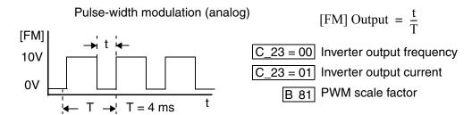
To calibrate the meter reading, generate a full-scale output (always ON) at terminal [FM]. Then use parameter B\_81(gain setting from 0 to 255) to adjust the corresponding full-scale reading of the meter. For example, when the inverter output frequency is 60 Hz, change the value of B\_81 so that the meter reads 60 Hz.
