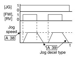
The type of deceleration used to end a motor jog operation is selectable by programming function A\_39. The options are:
