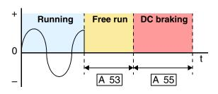
during deceleration below a frequency you can specify (A\_52). The braking power (A\_54) and duration (A\_55) can both be set. You can optionally specify a wait time before DC braking (A\_53), during which the motor will free run (coast).
