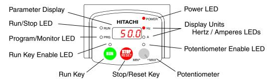
The display is used in programming the inverter's parameters, as well as monitoring specific parameter values during operation. Many functions are applicable only during the initial installation, while others are more useful for maintenance or monitoring.
