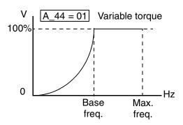
**Torque Boost** – The Constant and Variable Torque algorithms feature an adjustable *torque boost* curve. When the motor load has a lot of inertia or starting friction, you may need to increase the low frequency starting torque characteristics by boosting the voltage above the normal V/f ratio (shown at right). The boost is applied from zero to 1/2 the base frequency. You set the breakpoint of the boost (point A on the graph) by using
