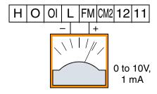
The signal characteristics of terminal [FM] in PWM configuration is shown below:
