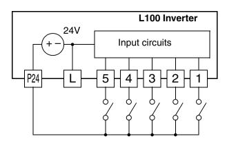
Sinking inputs, external supply
