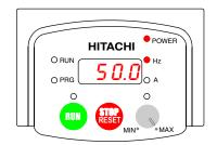
For the powerup test, monitor the motor speed indirectly by viewing the inverter's output frequency. The *output frequency* must not be confused with *base frequency* (50/60 Hz) of the motor, or the *carrier frequency* (switching frequency of the inverter, in the kHz range). The monitoring functions are in the "D" list, located near the top left of the "Keypad Navigational Map" on page 2–23.
