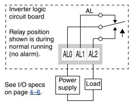
The alarm output terminals are connected as shown below (left) by default. The contact logic can be inverted as shown (below right) by using the parameter setting  $C_33$ . The relay contacts normally open (N.O.) and normally closed (N.O.) convention uses "normal" to mean the inverter has power and is in Run or Stop Mode. The relay contacts switch to the opposite position when it is in Trip Mode or when input power is OFF.
