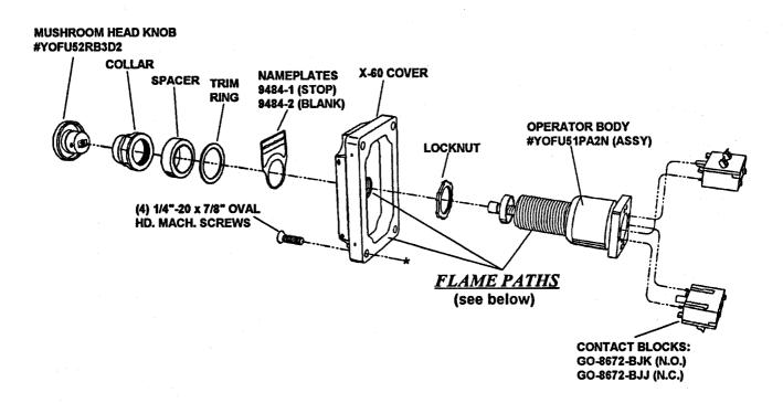
A FLAME PATH IS MACHINED ON BOX & COVER SUCH THAT A 0.0015" FEELER GAUGE WILL NOT ENTER THE JOINT MORE THAN 1/8" WHEN FULLY ASSEMBLED AND BOLTED. CARE MUST BE TAKEN THAT MACHINED SURFACES AND THREADED AREAS ARE NOT DAMAGED.
