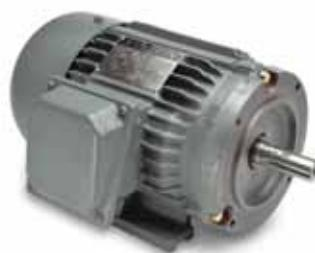
IronHorse 1800 rpm T-frame cast iron industrial duty motors are available from 1–300 hp, and TC-frame motors are available from 1–100 hp. Optional C-face kits are available for all IronHorse T-frame motors. All models have a TEFC frame and full length mounting feet.
