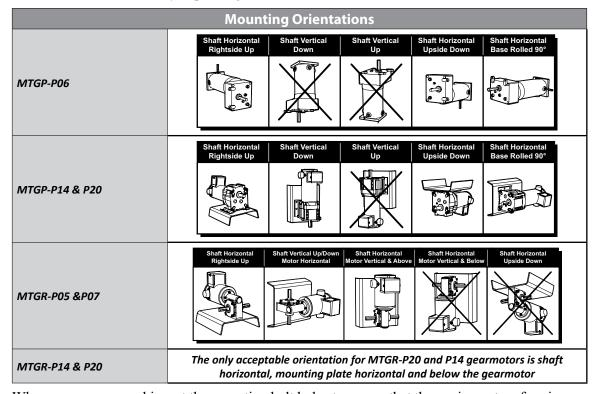
When necessary, use shims at the mounting bolt holes to ensure that the equipment surface is parallel to the gearmotor mounting surface. Use proper diameter bolts of the highest grade material available for the application, as shown on the dimension diagrams.
