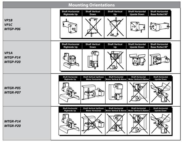
When necessary, use shims at the mounting bolt holes to ensure that the equipment surface is parallel to the gearmotor mounting surface. Use proper diameter bolts of the highest grade material available for the application, as shown on the dimension diagrams.
