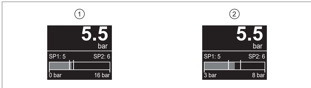
Fig. 32: Scaling of the bar graph display
