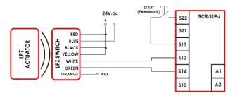
Multiple switches to SCR-31P-i Safety Relay (Viper series):
