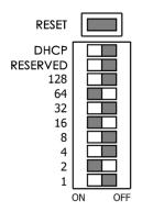
Out of the box the DIP switches are all set to the OFF position, if left unchanged the device will enter DHCP mode once powered and connected to the network.
