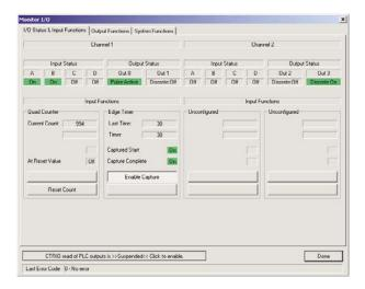
In the example above, the Current Count for Ch1/Fn1 Quad counter is 994. The Reset Count button can be used to reset the count to the configured Reset Value.
