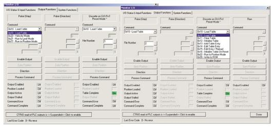
In the example above, Outputs 0 and 1 are configured for Pulse step and direction, Output 2 is configured to Preset mode assigned to Ch1/Fn1 (quad counter) and Output 3 is configured as Raw mode.
