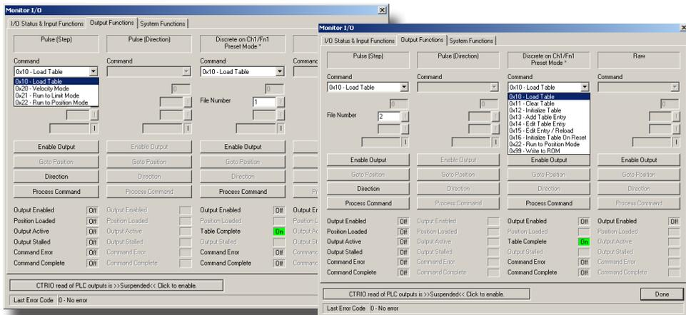
In the example above, Outputs 0 and 1 are configured for Pulse step and direction, Output 2 is configured to Preset mode assigned to Ch1/Fn1 (quad counter) and Output 3 is configured as Raw mode.
