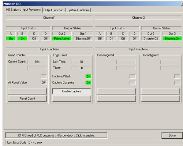
In the dialog panel above, the **Current Count** for Ch1/Fn1 **Quad Counter** is 994. The **Reset Count** button can be used to reset the count to the configured **Reset Value**.
