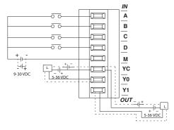
The module is configured, using CTRIO Workbench, to accommodate the user's application. The function of each input (counting, timing, reset, etc.) and output (pulse output, discrete output, etc.) is defined in the configuration of the module.
