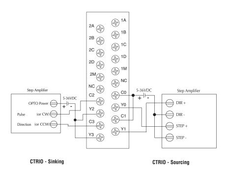
This example assumes that the Step Amplifier interface to be optocoupler LEDs (common anodes at the "OPTO Power" terminal) with internal current limiting resistors. This is a standard method; consult the step amplifier documentation to ensure that this method is applicable.
