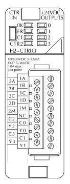
The H2-CTRIO(2) module has two independent input channels, each consisting of 4 optically isolated input points (1A–1D on common 1M and 2A–2D on common 2M). The inputs can be wired to either sink or source current. The module has 4 optically isolated output points (pts. Y0–Y3 with isolated commons C0–C3, respectively). The outputs must be wired so positive current flows into C(n) terminal and then out of the Y(n) terminal (see diagram
