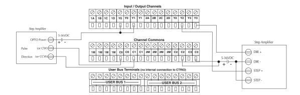
This example assumes that the Step Amplifier interface to be optocoupler LEDs (common anodes at the "OPTO Power" terminal) with internal current limiting resistors. This is a standard method; consult the step amplifier documentation to ensure that this method is applicable.
