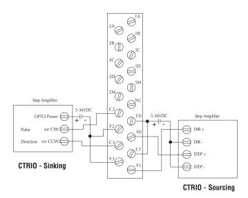
This example assumes that the Step Amplifier interface to be optocoupler LEDs (common anodes at the "OPTO Power" terminal) with internal current limiting resistors. This is a standard method; consult the step amplifier documentation to ensure that this method is applicable.
