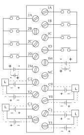
at left and the schematic on page 3-17). Remember that the internal jumpers can be used to connect the input commons or outputs/output commons together.
