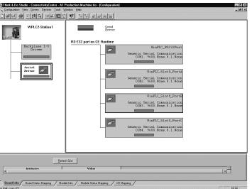
If you install additional Serial I/O modules at a later time, be aware that the order of the modules in the base determines their COM numbers. If you install a Serial I/O module between an existing Serial I/O module and the CPU, your port settings will remain the same, but the COM number will change.
