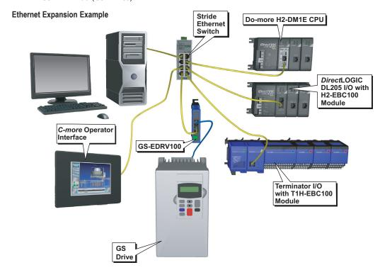
The Ethernet Expansion I/O network uses Category 5 UTP cables for cable runs up to 100 meters (328ft) with extended distances achieved through Ethernet switches.
