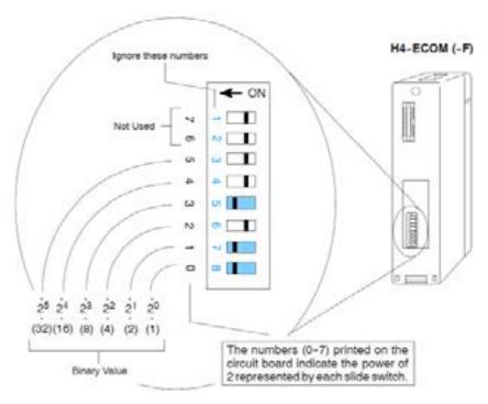
The Module ID equals the sum of the binary values of the slide switch set in the ON position. For example, if you set slide switches 0, 1, and 3 to the ON position, the Module ID will be 11. This is found by adding 8+2+1=11. The maximum value you can set on the DIP switch is 32+16+8+4+2+1=63. This is achieved by setting switches 0 through 5 to the ON position.
