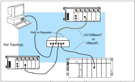
Hubs or repeaters can connect together to make it possible to connect more devices to the network or to extend the range of the network
