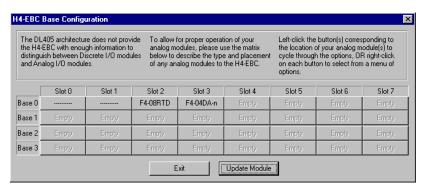
Once the correct part numbers appear for each of your analog modules, click the **Update Module** button to save the configuration into flash memory onboard the module. Leave the symbol "-----" wherever you have a digital module.
