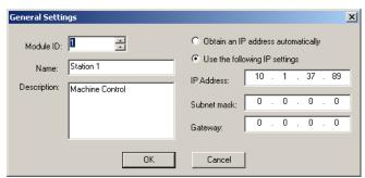
The General Settings box allows you to assign a **Module ID**. Module IDs must be unique for each EBC, but they do not have to be in sequence. The module's DIP switches must be set to zero to allow NetEdit3 to set a Module ID. Do not use address zero for communications.
