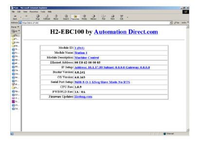
To configure the module, click on the desired parameter field. A new window will open, which are all described below and on the following page. Clicking the Back button will take you back to the main configuration screen shown above. Clicking the Send button writes the entry or change to the module's flash memory and clicking the Reset button reads the module's flash memory.
