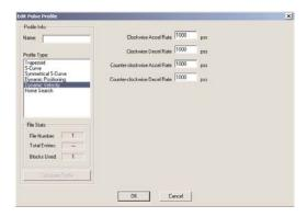
Clockwise Accel Rate: The clockwise rate at which the output will ramp up from 0pss to the target velocity that is specified in the CPU/controller memory register.
