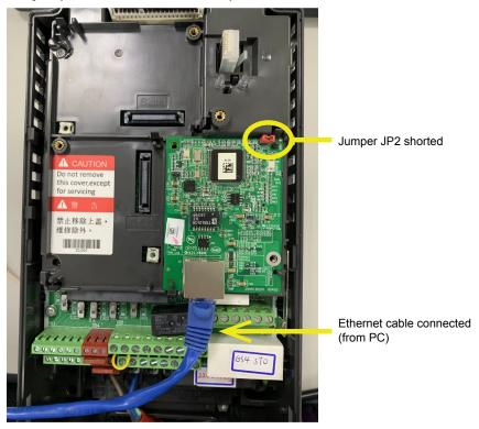
2) Set the PC IP address to **192.168.1.50** and connect the PC and the GS4 comm card with the ethernet cable (as shown in step #1).
